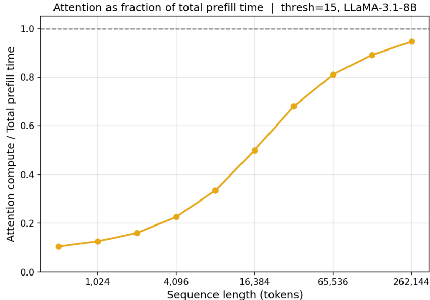
Figure 12: Attention compute as a fraction of total prefill time for DeltaAttention at threshold 15 on LLaMA-3.1-8B. At short sequences attention is a small fraction of total time; at 262K tokens it accounts for 95% of the forward pass.
